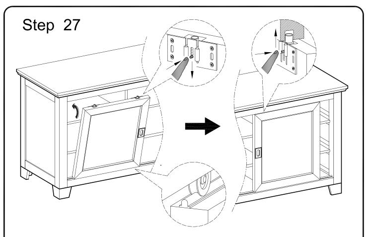
Insert the doors into the console by pulling down the upper door pins and carefully placing the door wheels over the slide in the bottom panel. Secure the doors into place by pressing the upper door pins into the groove in the top panel.
